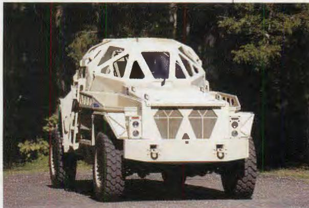
a blast bucket that helps deflect the energy of exploding mines. The result of this research is called the ULTRA AP. Office of Naval Research will now test the ULTRA AP to glean it for ideas that may be of use in future GI vehicles, and it is anticipated more will be built for field tests with mines and roadside bombs as well. *Photo: U.S. Navy, by John E. Williams*
