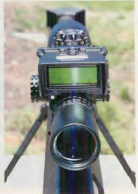
*Pre-programmed with many loads, the BORS has a tiny TV screen for instant readout of elevation adjustment to make first-shot hits at extended ranges.*
