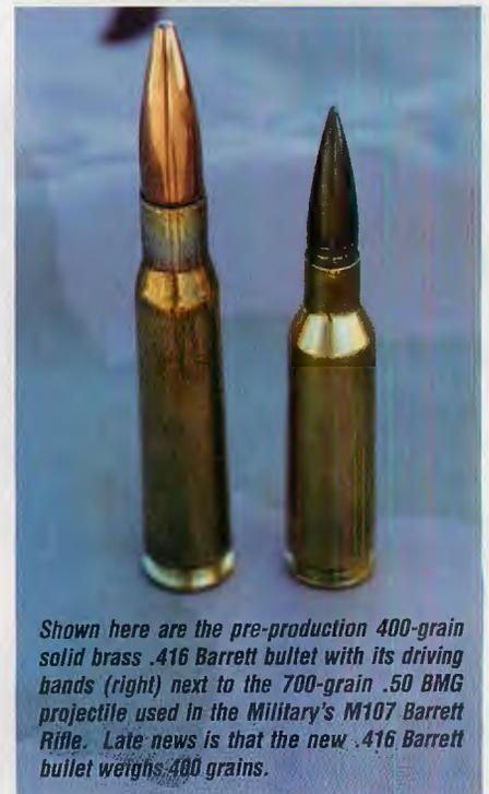
Shown here are the pre-production 400-grain solid brass .416 Barrett bullet with its driving bands (right) next to the 700-grain .50 BMG projectile used in the Military's M107 Barrett Rifle. Late news is that the new .416 Barrett bullet weighs 400 grains.
