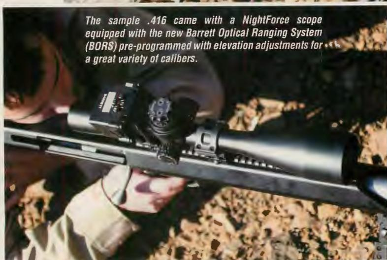
*The sample .416 came with a NightForce scope equipped with the new Barrett Optical Ranging System (BORS) pre-programmed with elevation adjustments for a great variety of calibers.*
