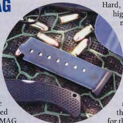
Hard, ACT-MAG had a high quality 1911 magazine, which Wayne Novak wanted to adopt, but first Wayne made modifications to the feed lips for optimum reliability. He also made a subtle change to the angle of the cut for the magazine catch, for better release during
